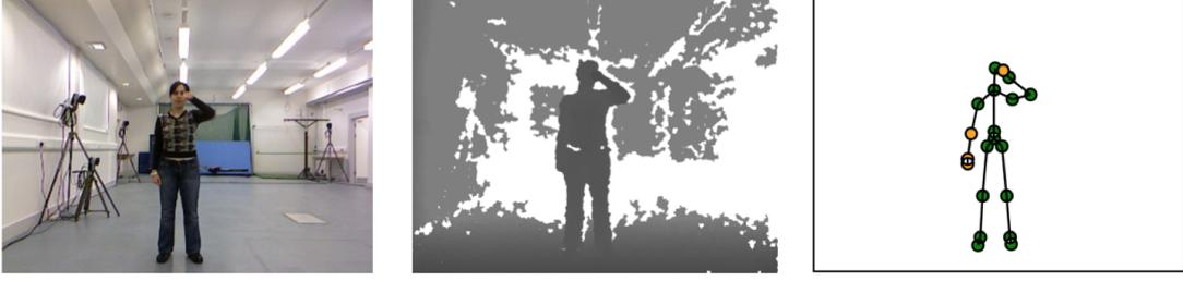
Figure 2.3: A colored image with its associated depth image and extracted skeleton. [3]
